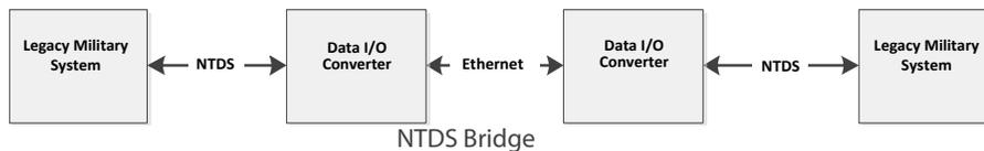
Similar to the NTDS Bridge, the ATDS Bridge connects and extends the cable run between ATDS equipment. It consists of two Data I/O Converters that communicate over Ethernet.
